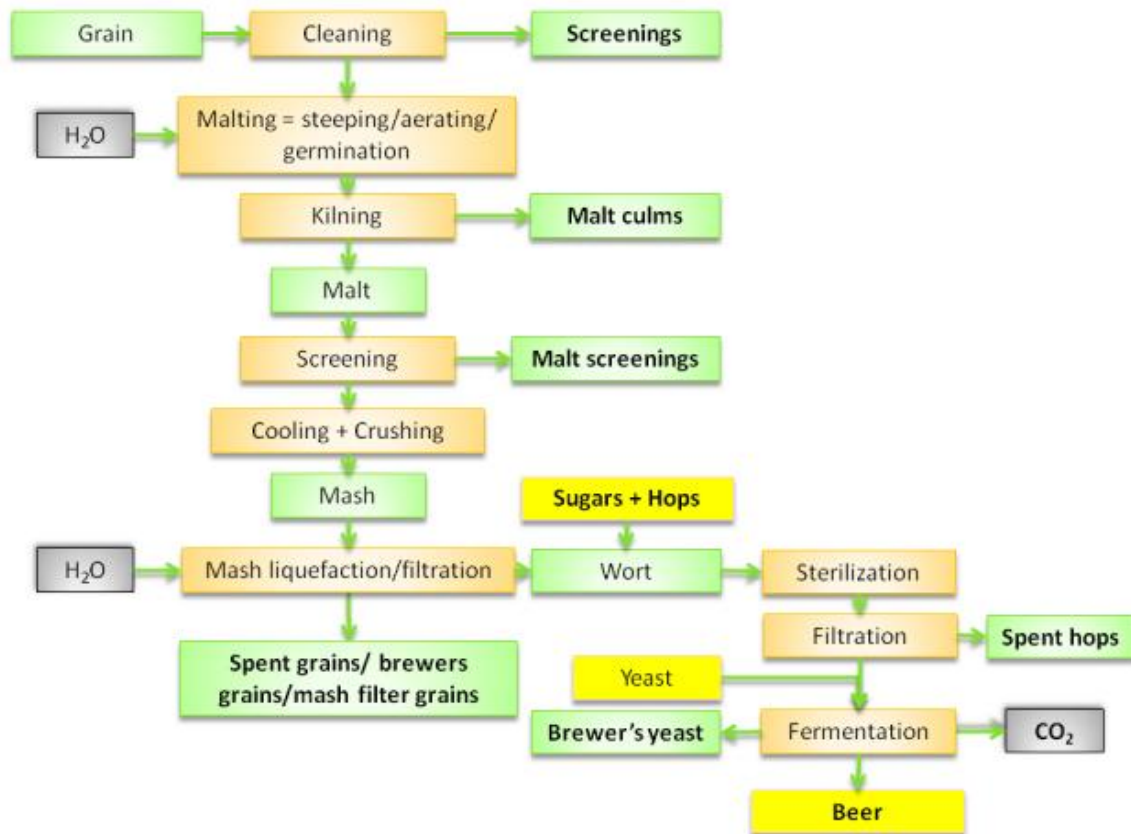
Figure 38. Process scheme of beer brewing process (Heuze et al., 2017)
