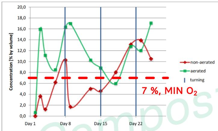
Picture 20: Comparison of the  $O_2$ -contents of the bio waste windrows
