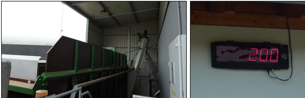
Picture 1: Feeder for bulky substrates with included weighing unit and big display also directly on the device so staff has control when loading the feeder.
